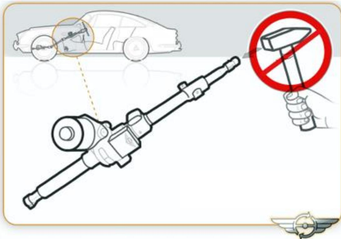
Never strike the input shaft with an object during or after assembly. This can adversely affect the sensors.
