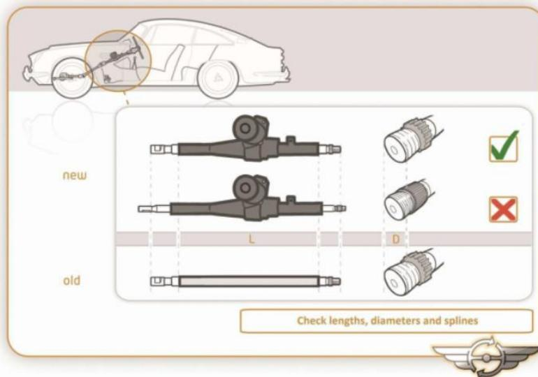
In the car industry its common to have some small tolerances in spline connections. In very exceptional cases connecting a new shaft from the EZ-unit in the original (old) U-joint could cause a tight fitting. This is sometimes relatively easy to solve by sanding only about 0,2mm (0,007 inch) in the inner part of the U-joint and also the spline on the output shaft on the EZ-unit.
