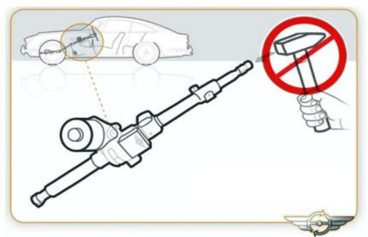
Never strike the input shaft with an object during or after assembly. This can adversely affect the sensors.
