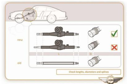
In the car industry its common to have some small tolerances in spline connections. In very exceptional cases connecting a new shaft from the EZ-unit in the original (old) U-joint could cause a tight fitting. This is sometimes relatively easy to solve by sanding only about 0,2mm (0,007 inch) in the inner part of the U-joint and also the spline on the output shaft on the EZ-unit.
