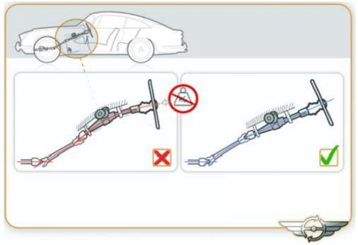
The steering system must always be properly aligned and mounted without tension.
